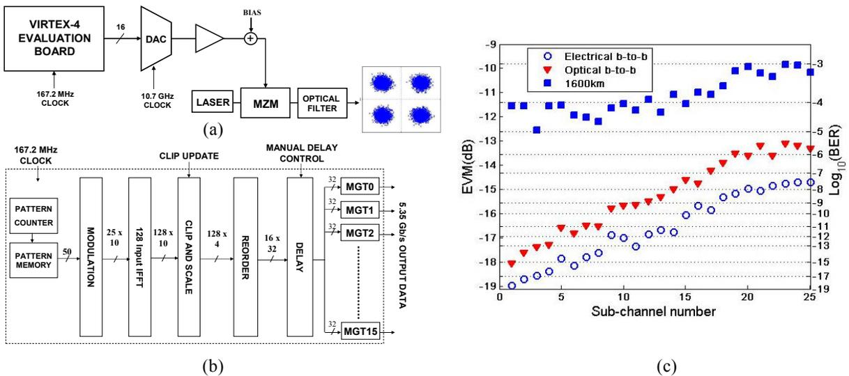
Fig. 1 (a) OFDM transmitter design (b) DSP block functions (c) EVM & BER per sub-channel [1]
