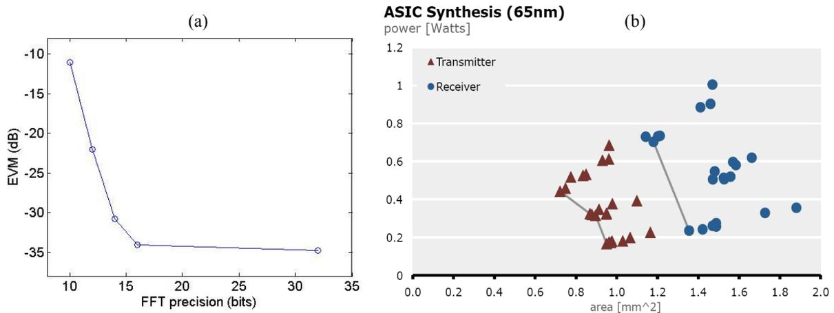
Fig. 2 (a) Received signal EVM against FFT resolution (b) Power vs. chip area for various transmitter/receiver designs [8]
