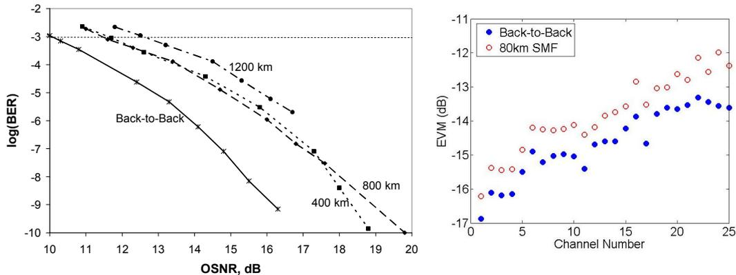
Fig. 2 Left BER versus OSNR for 10.7 Gb/s EPD signals [3], Right: Measured EVM for 8.35 Gb/s OFDM signals
