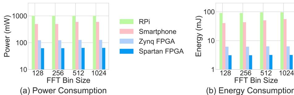
Figure 5: Comparison of power and energy consumption of our FPGA, Raspberry-Pi and smartphone based sensors.
