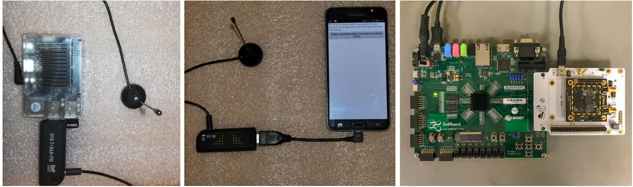
(a) Raspberry-Pi based sensor      (b) Smartphone based sensor      (c) FPGA based sensor
