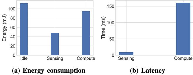
Figure 2: Energy consumption and latency of each unit of a Raspberry-Pi based spectrum sensor.
