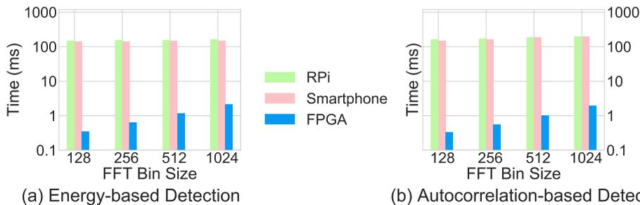
**Figure 4: Comparison of latency of the compute unit of our FPGA, Raspberry-Pi and smartphone based sensors.**
