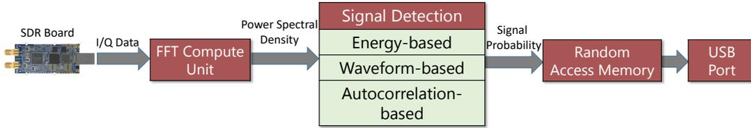
Figure 1: An overview of our FPGA-based spectrum sensor.
